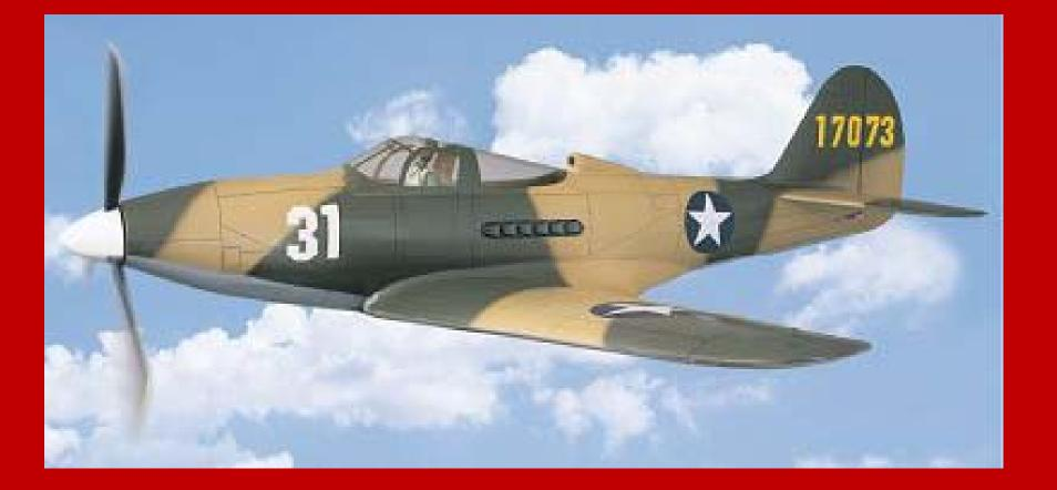
When the men of the 332nd Fighter Group arrived in Taranto, Italy, they were initially assigned the task of coastal patrol flying an obsolete aircraft the Bell P-39 Airacobra. The Airacobra was slow compared to first line German and Italian fighters. Its main claim to fame was the 37mm cannon that fired through the propeller spinner.
